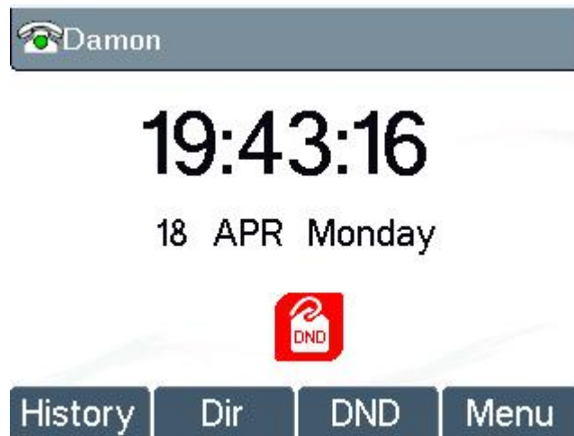
Figure 57 - DND Enabled on All Lines
